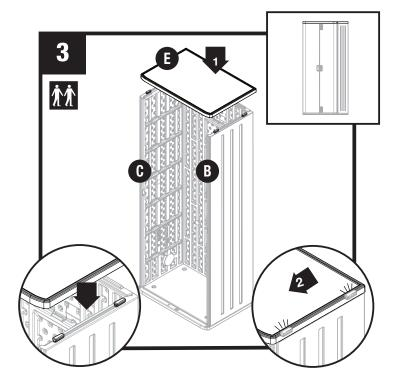
Align slots on top panel (E) with tabs on side panels (C/B). Lower top panel and lock in place by sliding panel towards front. Top will overhang front slightly.
