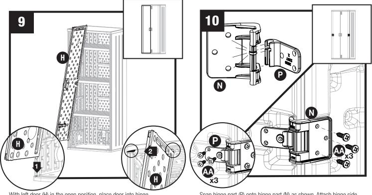
With left door (H) in the open position, place door into hinge receptacle on bottom left of cabinet. Insert hinge pin under top panel and slide to the left into hinge receptacle. Repeat with right door (G).
