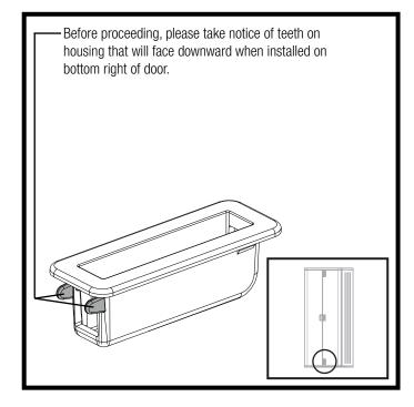
Insert door latch housing (K) into bottom right door (G) and snap into place. Insert door latch (J) into door latch housing. Push latch pin down so it is fully seated in latch housing. Push down with force until you hear a snap. Slide latch up and down to confirm it slides properly.
