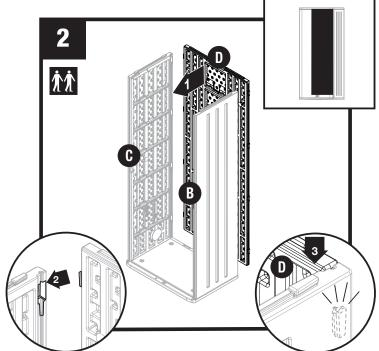
Align and engage tabs on back panel (D) with slots on side panels (C/B). Push panel D down to lock in place.
