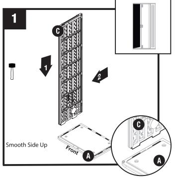
Align tabs on left side panel (C) with slots on bottom panel (A). Lower side panel into slots and lock in place by sliding panel towards front. Repeat with right side panel (B).
