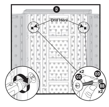
Using a 1/2 drill bit, drill through the two provided locations on Back Panel (D). Place cabinet in desired location. With a pencil mark the hole locations on the wall, and drill through the wall with 1/2 drill bit.
