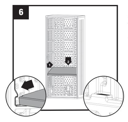
Tab on shelf must engage with slot on inside panel for each shelf. Push side panels inward to engage.
