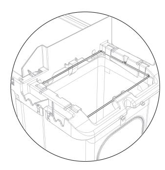
Lower garbage bag rim (R) and insert into two center slots provided. Guide rim into position. Repeat with right rim. **Note:** Rims can be put on both sides.
