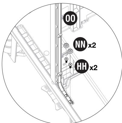
Attach (00) to bottom using two screws (HH) and two caps (NN). Repeat on right side. **Note:** Do Not attach top of tube (00) to lid until after step (21). Use a mallet to attach caps (NN).
