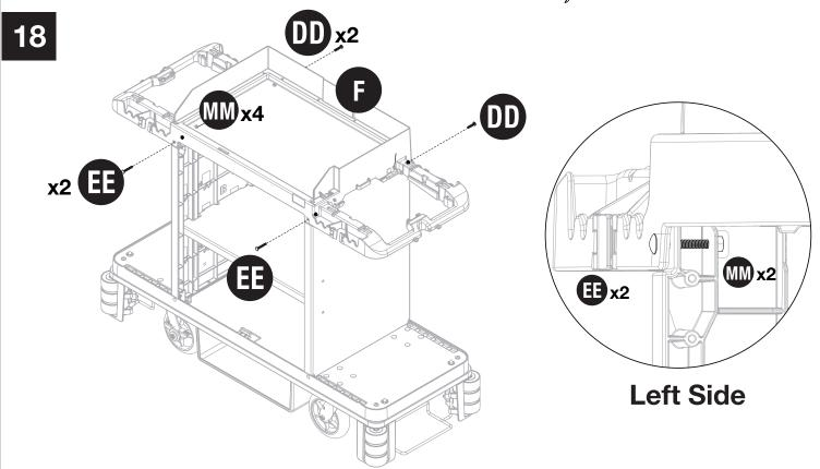
To attach lid (F) insert screw (EE / DD) through lid and attach nut (MM) from underneath lid. Note: Use supplied wrench \*
