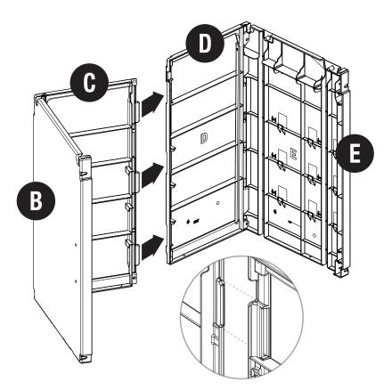
Insert Left back panel tabs (B/C) into slots on right back panel (D/E) on an angle and push together.
