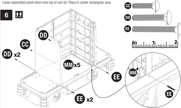
Attach sides to cart in four corners and center using five screws (CC /DD / & EE) and five nuts (MM).
