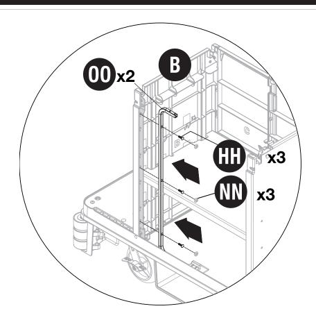
Insert tube (OO) into pocket in (B) and attach using three screws (HH) and three caps (NN). Repeat on right side. Use a mallet to attach caps (NN).
