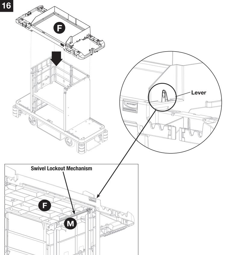
Lower top (F) to top of cart. Make sure the upper Swivel Lockout Bar (M) stays in position. The red lever should remain vertical so it fits properly through the hole on the lid (F). Lid (F) should cover part of upper Swivel Lockout Bar (M) on the inside.
