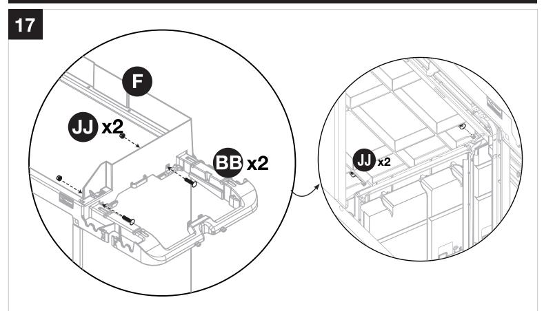
To attach lid (F) insert bolt (BB) through hole on side of cart and attach from underneath lid using nut (JJ). Repeat other side. Note: Close up views have had shelf taken out for clarity. **Note: Use supplied wrench** \*\*
