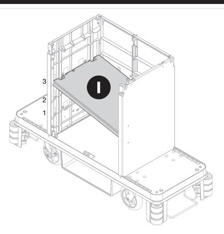
Insert shelf (I) into cart at an angle in one of three positions.
