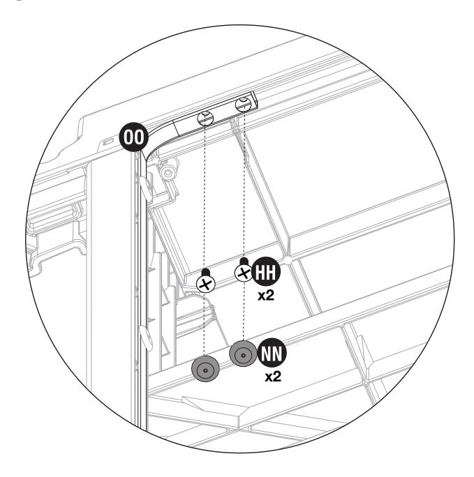
Attach tube (OO) to top using two screws (HH) and two caps (NN). Use a mallet to attach caps (NN). Repeat other side.
