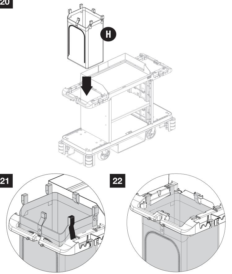
Lower garbage bag (H) through frame of cart. Unsnap and feed through the six slots on frame. Re-snap the bag once strap is through each slot. **Note:** Bag can be switched to other side if necessary.
