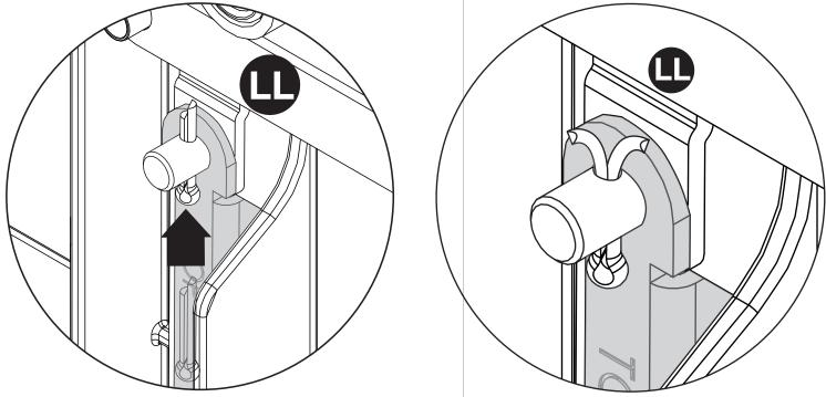
Insert two holes on Swivel Lockout Mechanism (M) onto two pegs on side panel hole also stamped "top". Slide all the way to the back. Attach by placing cotter pin (LL) through hole. Fold Cotter pin over using a needle nosed pliers. Repeat other side.
