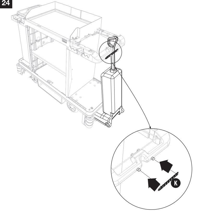
Attach rubber strap (K) over two knobs on side of cart to secure vacuum cleaner. Vacuum cleaner not included.
