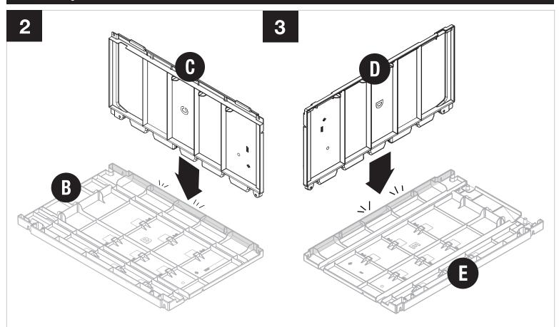
Insert back left panel (C) into left side panel (B) until secure. Insert back right panel (D) into right side panel (E) until secure.
