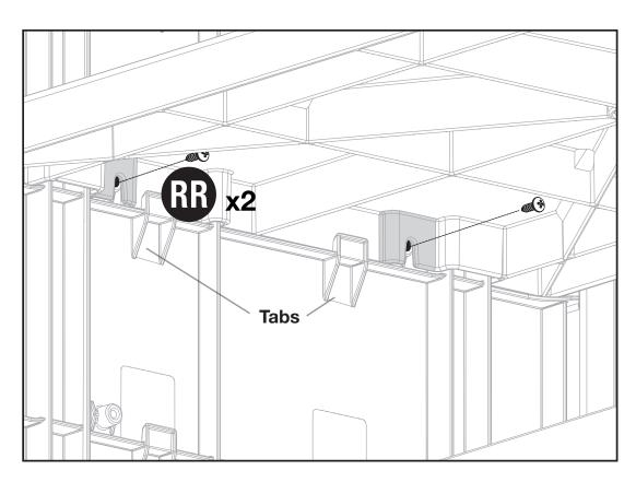
Push down till sides of shelf engage with tabs on sides of cart. Attach shelf to sides using two screws (RR). Repeat other side.
