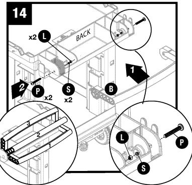
Attach handle (B) to cart using two bolts (P), two lock washers (S) and two nuts (L). **Note:** There are three different handle positions.
