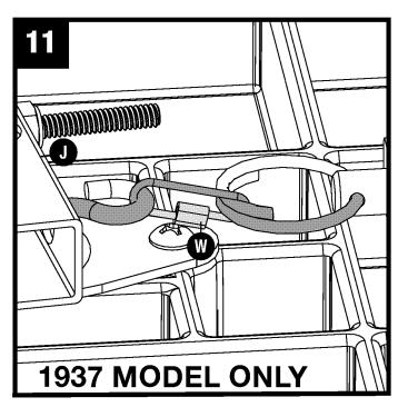
Thread clip style, lanyard loop, (W) onto key ring. Clip other end of loop onto hook. Repeat other side. **Note:** Ring should already come attached to caster.
