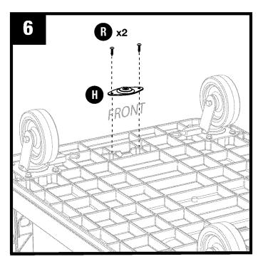
Attach Pivot plate (H) to front of cart using two screws (R).
