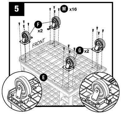
Attach each caster (F/G) to bottom (E) using sixteen screws (M).**Note:** Casters with ring should be placed on the front. Front has beveled corners. Make sure ring is in horizontal position when insalling casters. Ring always faces inside!
