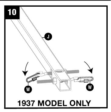
Thread lanyard loop (W) onto hooks connected to (J). **Note:** Make certain nuts on opposite side of hooks are completely fastened.
