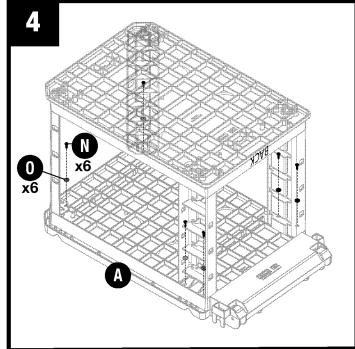
Attach each vertical leg to top (A) using six washers (O) and six screws (N).
