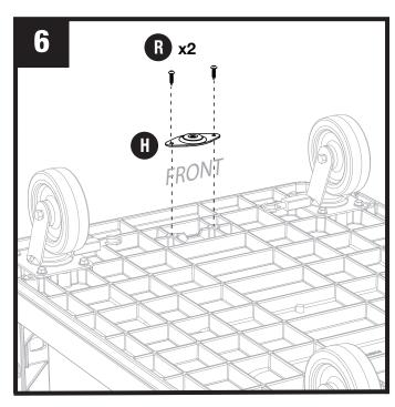
Attach Pivot plate (H) to front of cart using two screws (R).
