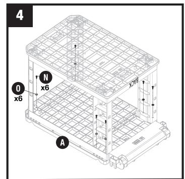
Attach each vertical leg to top (A) using six washers (O) and six screws (N).
