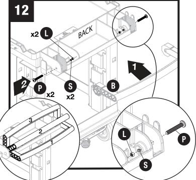
Attach handle (B) to cart using two bolts (P), two lock washers (S) and two nuts (L). **Note:** There are three different handle positions.
