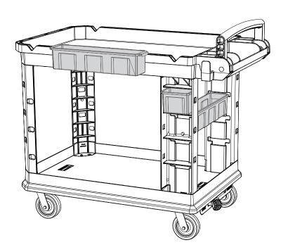
Insert rim of small bin on inside of leg (D) or on outside rim of cart as shown on top image. Bin can fit in five positions. Insert rim of large bins inbetween legs (D) or rim of large bin can hang off either side of upper platform (A).
