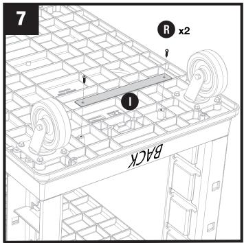
Attach slide plate to back of cart using two screws (R). **Note:** Back of cart has handle.
