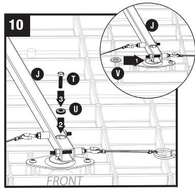
Slide washer (V) under (J) and attach to bar using nylon washer (U) and bolt (T).
