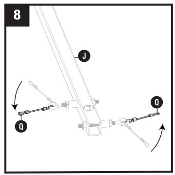
Thread lanyard (Q) onto hooks connected to (J). **Note:** Make certain nuts on opposite side of hooks are completely fastened.
