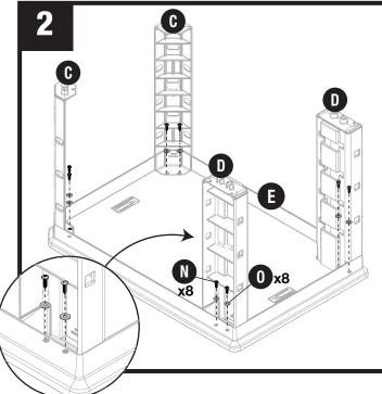
Lower each support (C/D) to bottom base (E). Peg on each leg must be inserted and pushed in hole on base. Smooth side of bottom base (E) must be up.
