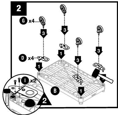
Insert Caster (G) into corner hole in bottom of tray (B). Repeat for each corner of tray. Evenly tap each wheel with mallet until fully seated and secure. Turn tray right side up.
