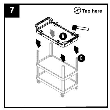
Lower top tray (B) and insert on top of corner posts (E). First, push down all four corners evenly by hand. Then, evenly tap with mallet on locations indicated until fully seated and secure.
