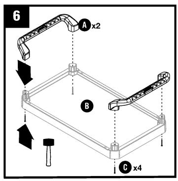
Insert handle (A) onto tray (B). Gently tap each handle corner with mallet to secure handle (A) to tray (B). Attach using 4 screws (C).
